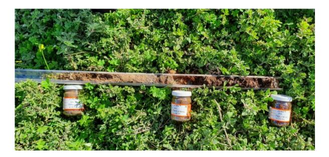
Photo 4. An example of the geology at SB06, showing sand, gravel and clay material
