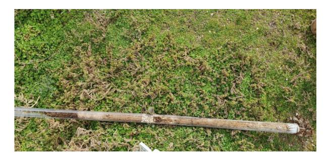
Photo 6. An example of the geology at SB03, showing sand, gravel and clay material. Also showing the gravel layer In the middle of the push tube where a plastic layer was also present
