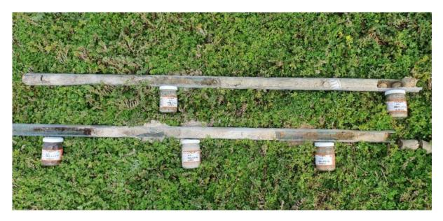
Photo 5. An example of the geology at SB02, showing sand, gravel and clay material
