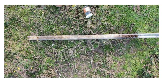
Photo 3. An example of the geology at SB05, showing sand, gravel and clay material
