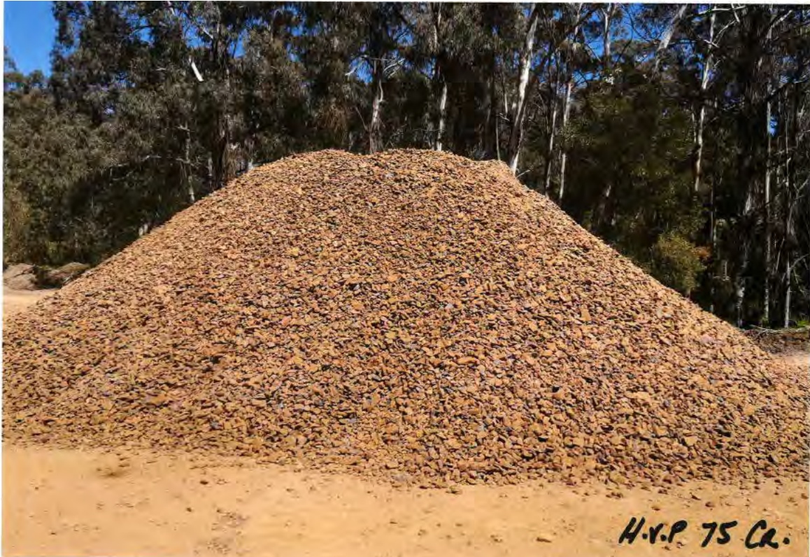
Stockpile of 75 mm Non-Descript Crushed Rock. Photo provided by Ross Kennedy.
