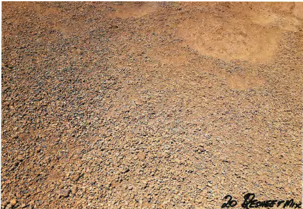
Stockpile of 20 mm Non-Descript crushed rock – ‘Resheet Mix’. Photo provided by Ross Kennedy.
