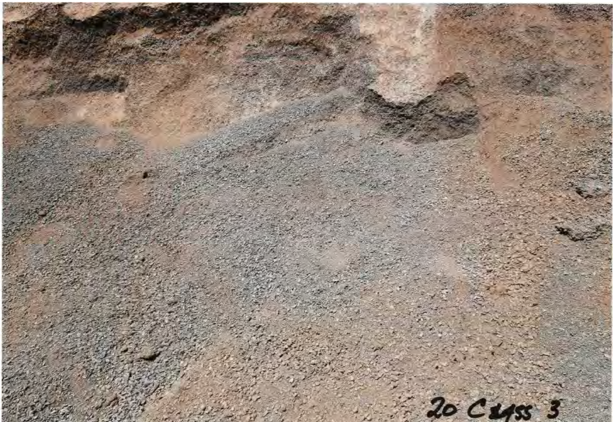
Stockpile of 20 mm VicRoads Class 3 crushed rock. Photo provided by Ross Kennedy.
