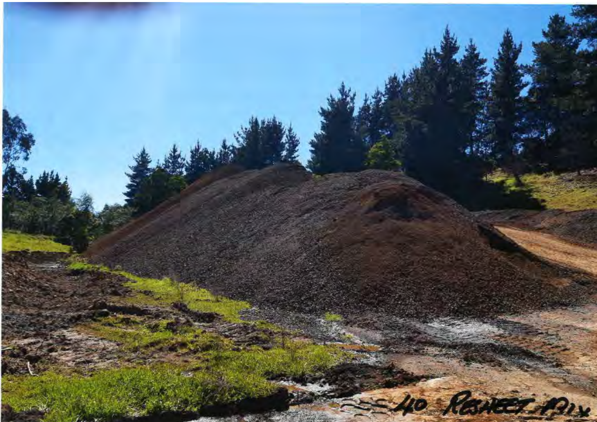
Stockpile of 40 mm Non-Descript crushed rock – ‘Resheet Mix’. Photo provided by Ross Kennedy.
