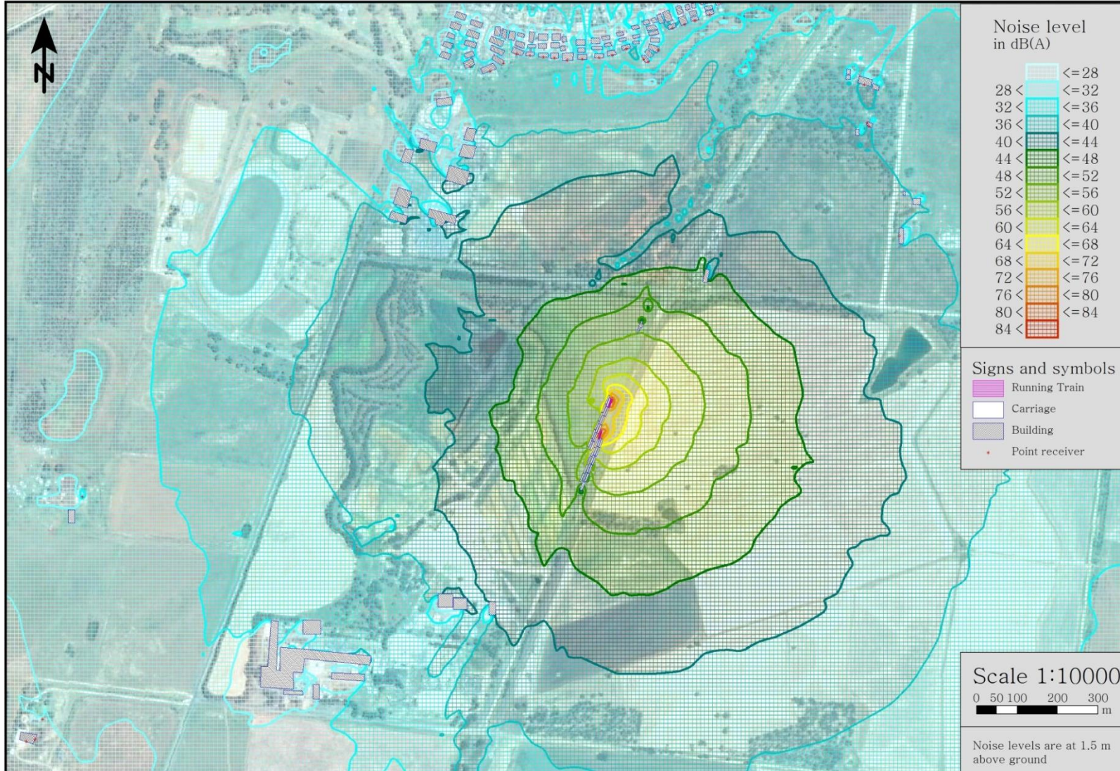
FIGURE B-1 PREDICTED NOISE CONTOURS OF THE MADDINGLEY STABLING YARD WITH TWO N-CLASS TRAINS RUNNING
