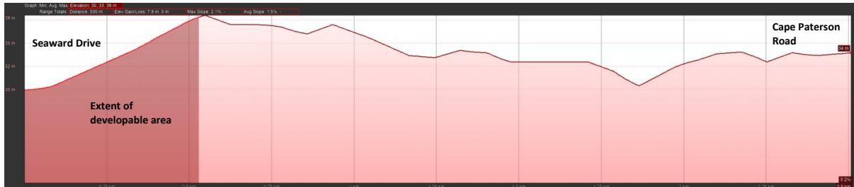
Figure 66 – CP Rd 1 - Exaggerated elevation profile – boundary located to south of topographic high point at approximately 39m AHD (Source: Google Earth).
