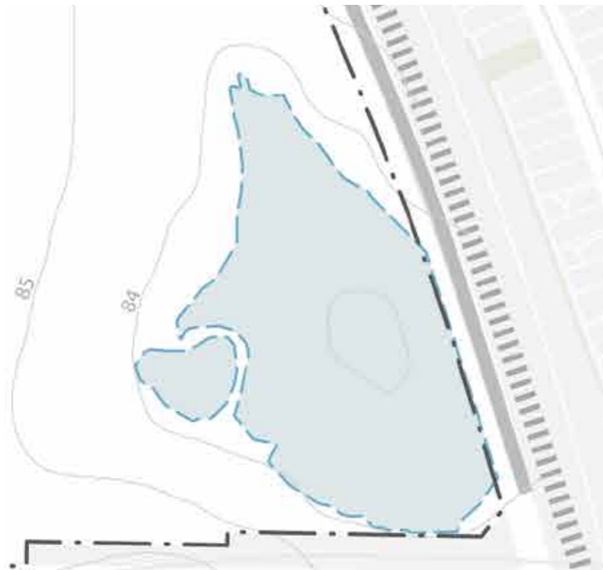
Extent of flooding as it currently exists for 1 in 100 year event. The existing flood level is 83.88m to AHD.
