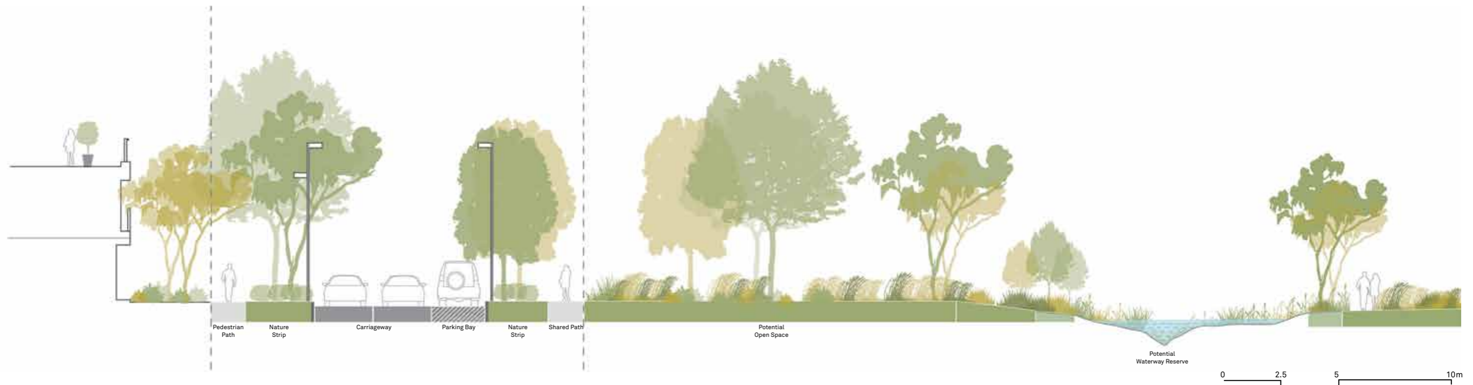
Typical Section through Private Allotments, Local Access Street, Public Open Space and St Albans West Drain indicating planting opportunities
