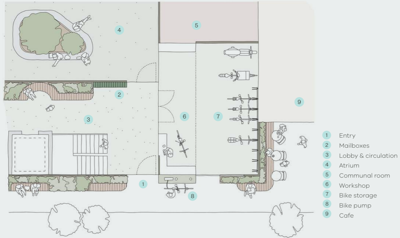
Figure 2.3 Activated communal spaces create opportunities for incidental interactions. These include circulation spaces such as lobbies, stairs and corridors, with connections to residents' amenity spaces. Building a dynamic relationship between the lobby, external residents' spaces and shared uses is encouraged.
