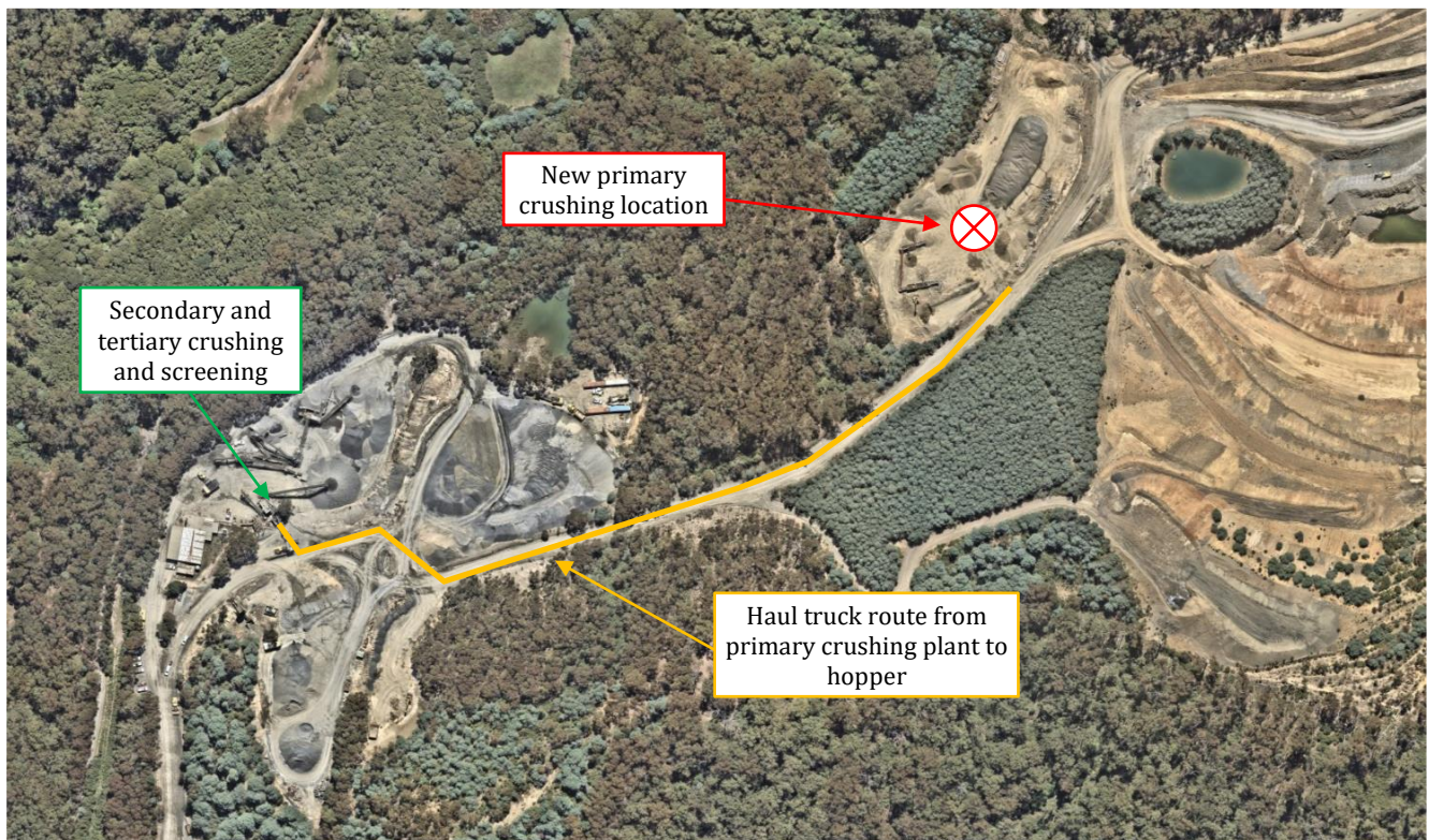
Figure 8: Aerial image including new location of primary crushing plant and haul truck route
