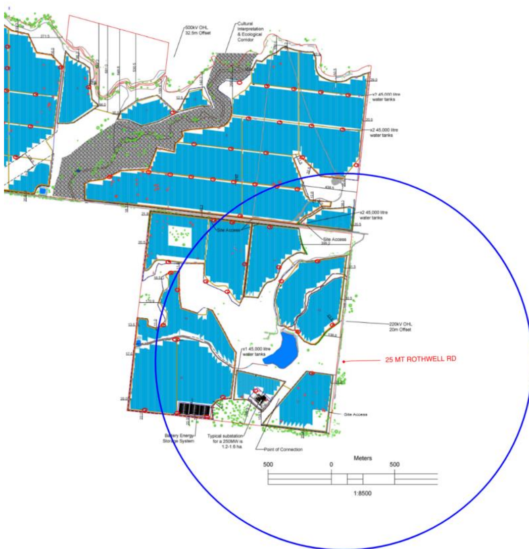
Figure 4 Inverters within the blue circles will require acoustic barriers
