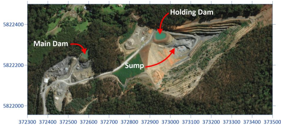
FIGURE 8.3 WA375 Water Storage Locations
