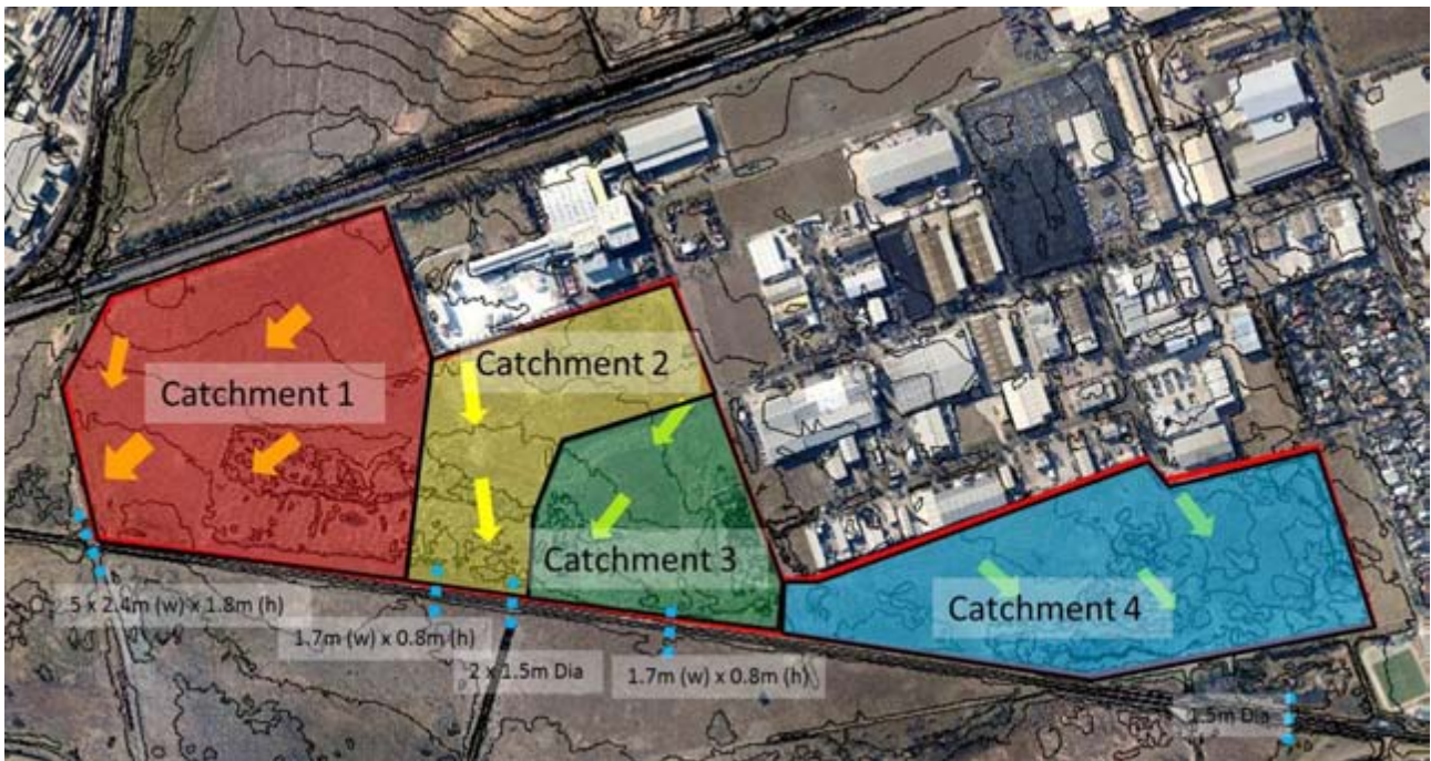
Figure 2: Existing catchment, flow directions and culverts
