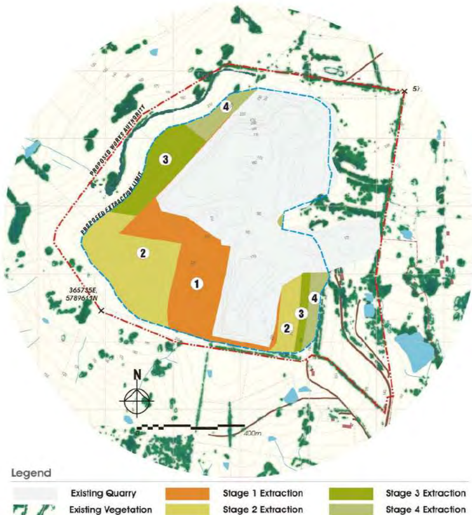
FIGURE 4-1 GENERAL EXCAVATION STAGING PLAN
