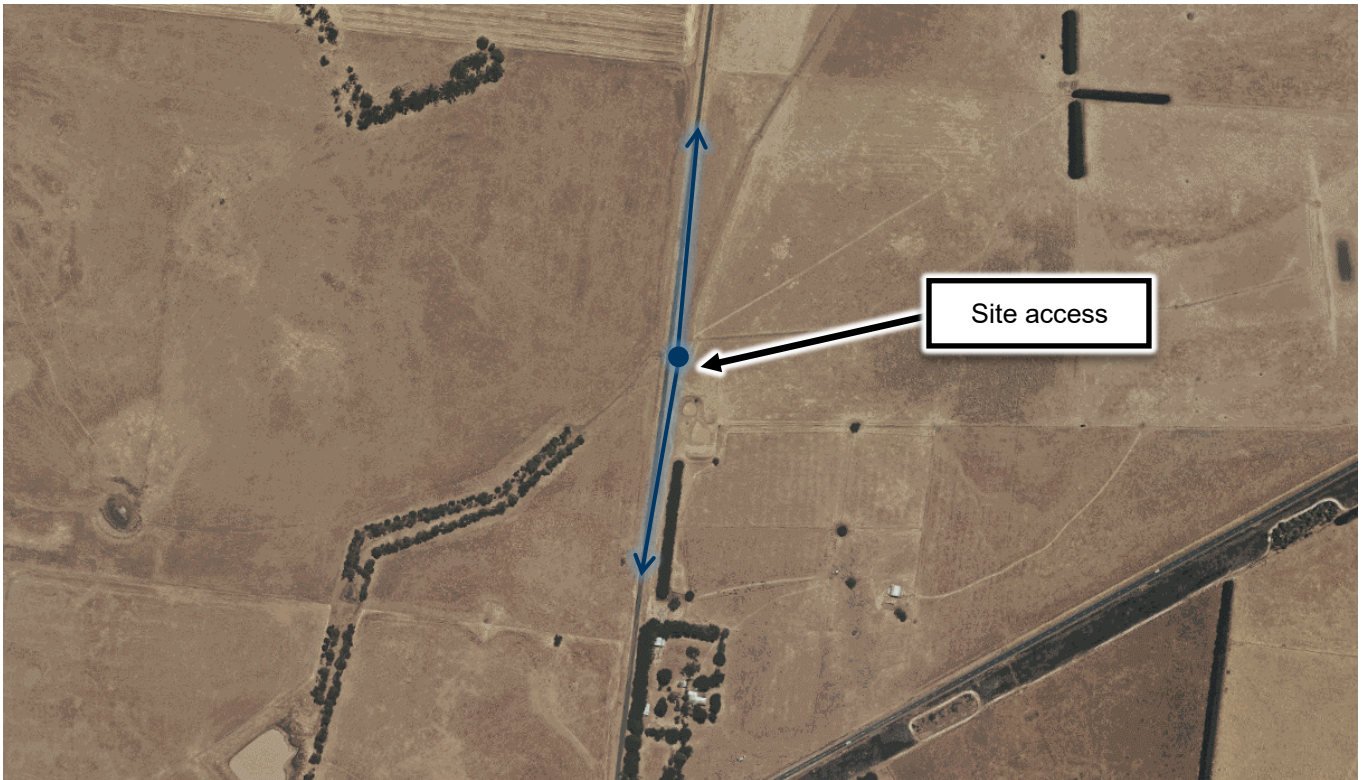
Figure 15 Sight distance at Six Mile Lane access
