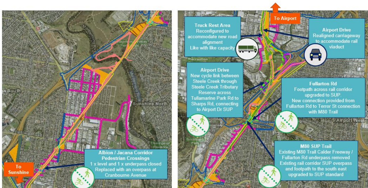
Figure 5-1: Locations of Permanent Changes to the Wider Transport Network Following MAR under Corridor Section
