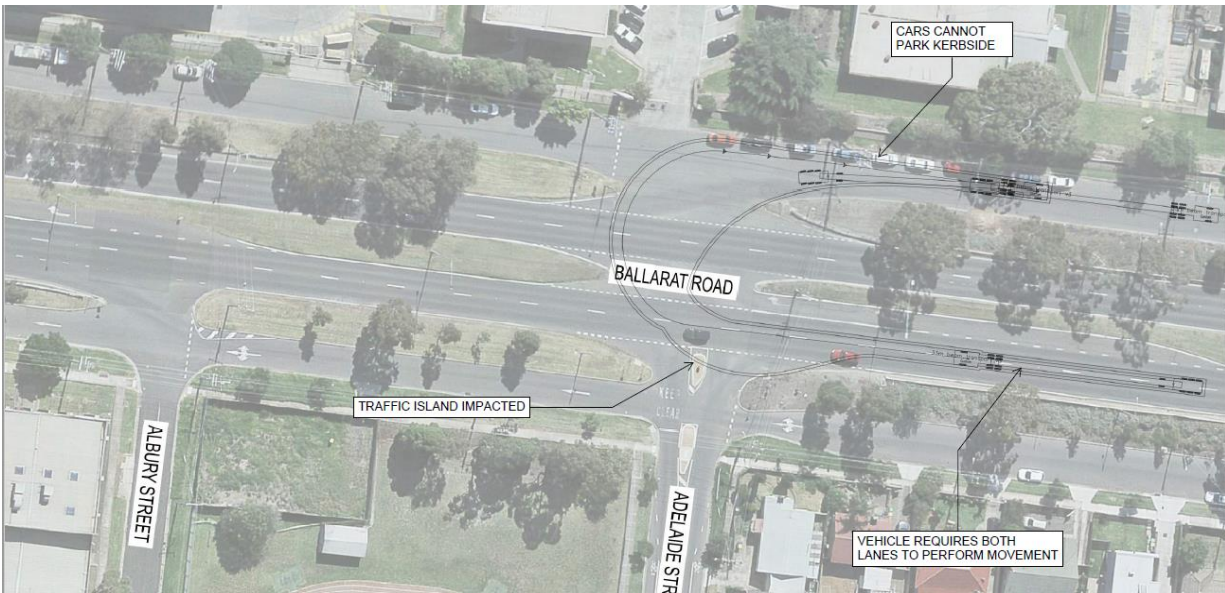
Figure 8-9: Over Dimensional Swept Path Assessment – Ballarat Road to Ballarat Road Service Road
