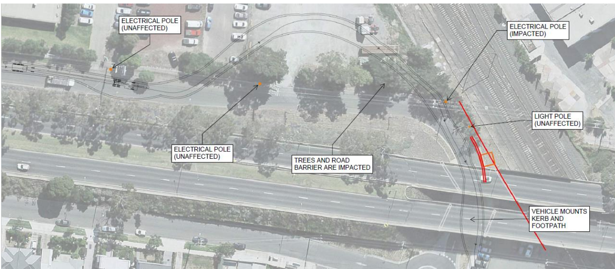
Figure 8-10: Over Dimensional Swept Path Assessment – Ballarat Road Service Road into Albion Station Car Park
