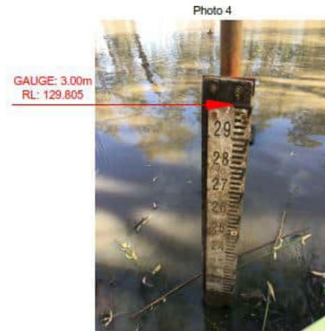
Figure 3-3: Potential Movement at Chamber's Gauge Post
