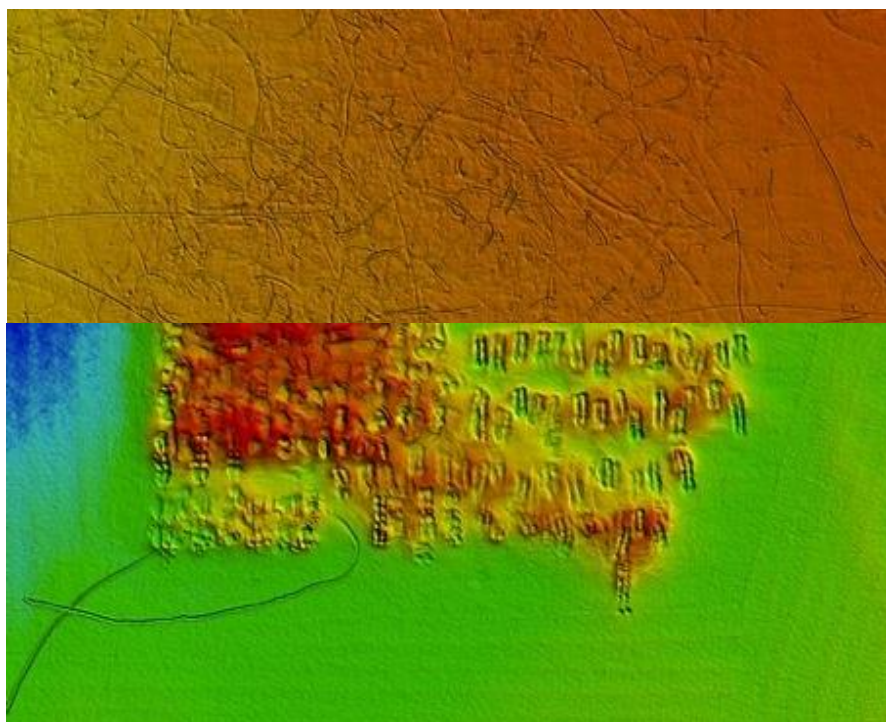
Figure 25 Multibeam bathymetry showing gouging scars on the seabed in an anchorage zone (top) and DMG mounds and scraping of spoil placement device in the southeast of the Bay (bottom).
