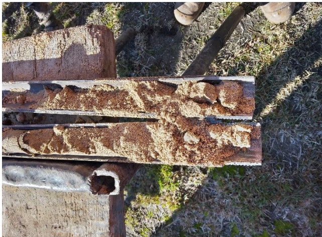
Photo 16: Borehole 3 SPT sample at 4.0m XW Sandstone.
