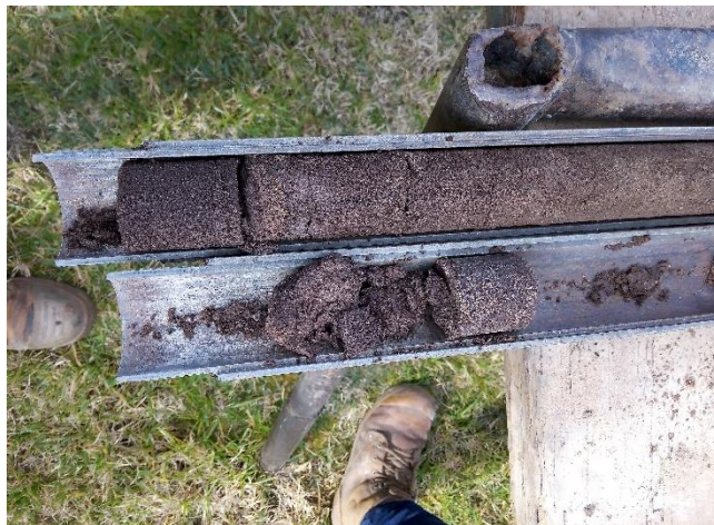
Photo 28: Borehole 6 SPT sample at 2.5m, Silty SAND.
