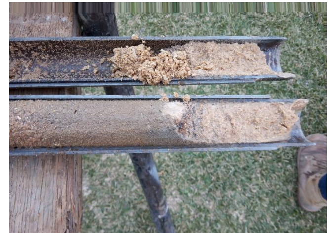
Photo 6: Borehole 1 SPT sample at 2.50m Silty SAND.
