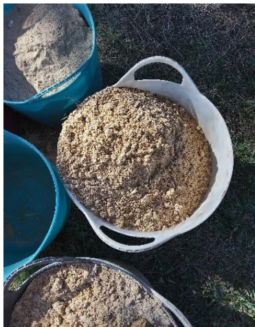
Photo 10: Soil spoil from Borehole 8. Silty SAND.
