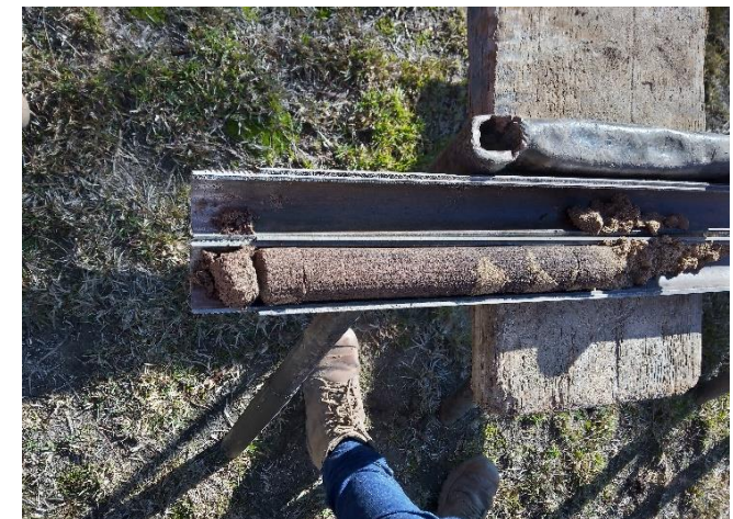
Photo 18: Borehole 4 SPT sample at 1.0m, Silty Sand FILL.
