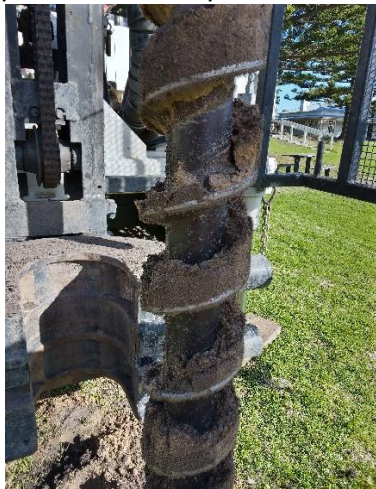
Photo 10: Soil profile of borehole 2, Silty SAND.
