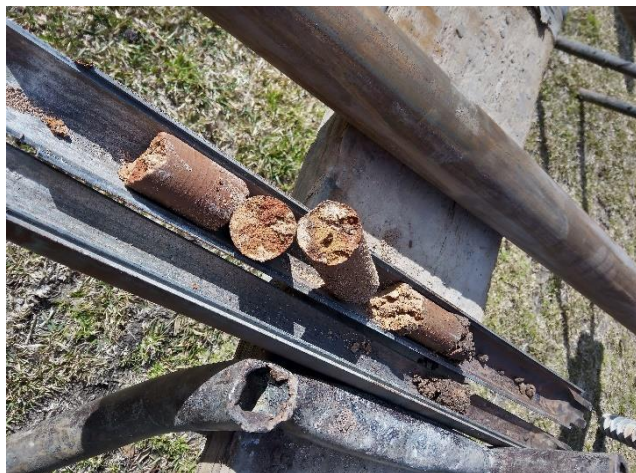
Photo 23: Borehole 5 SPT sample at 2.5m.
