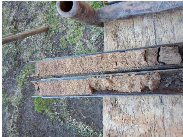
Photo 14: Borehole 3 SPT sample at 1.0m, Silty SAND.
