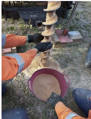
Photo 4: Borehole 7 spoil. Silty SAND.
