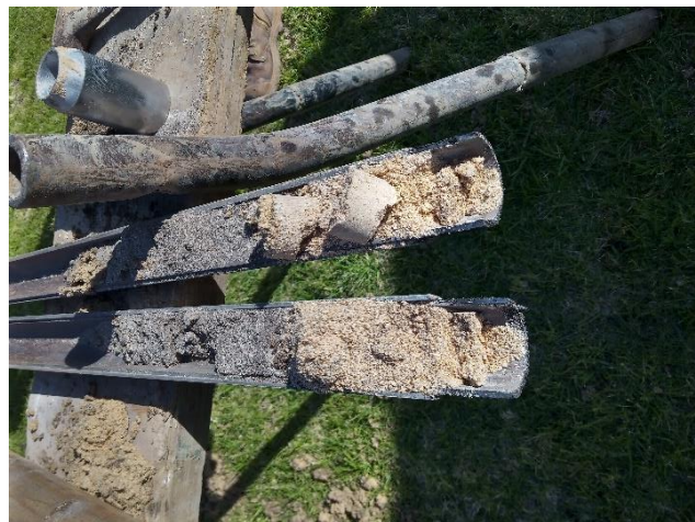
Photo 11: Borehole 2 SPT sample at 2.5m, Silty SAND.
