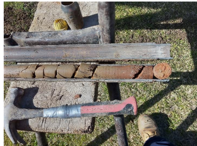
Photo 29: Borehole 6 SPT sample at 4.0m, Clayey SAND/Sandy CLAY.
