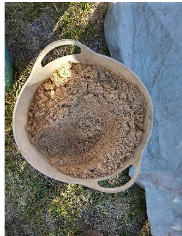
Photo 5: Soil spoil of Borehole 7. Silty SAND.
