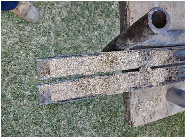
Photo 4: Borehole 1 SPT sample at 1.0m Silty SAND.
