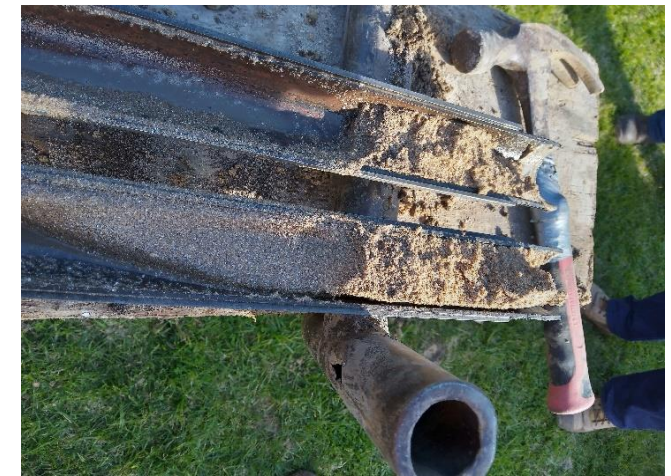
Photo 12: Borehole 2 SPT sample at 4.0m, very saturated Silty SAND.
