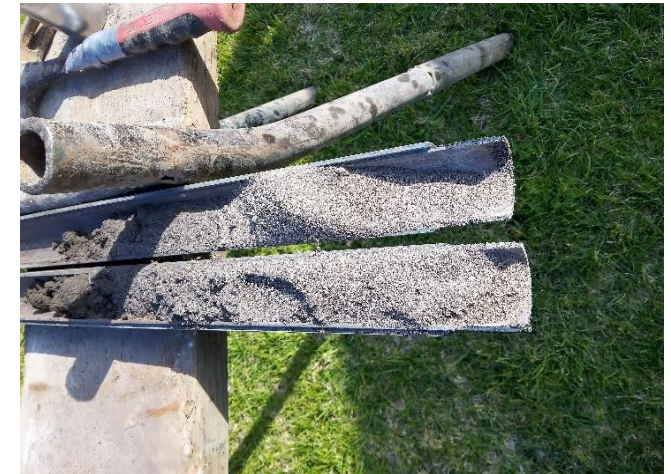
Photo 9: Borehole 2 SPT sample at 1.0m, Silty Sand FILL.
