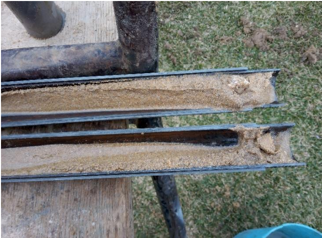
Photo 7: Borehole 1 SPT sample at 4.0m, very saturated Silty SAND.
