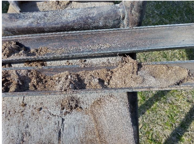
Photo 26: Borehole 6 SPT sample at 1.0m, Silty SAND.
