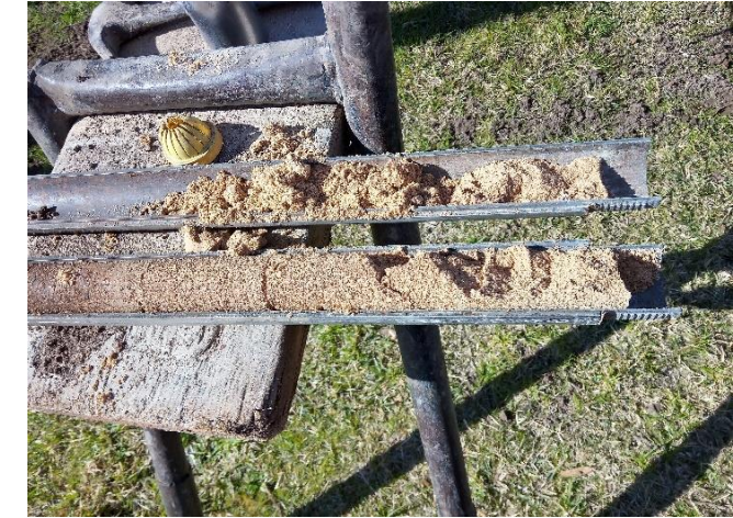
Photo 12: Borehole 6 SPT sample at 5.5m, Clayey SAND. © 2021 LR Pardo & Associates Pty Ltd
