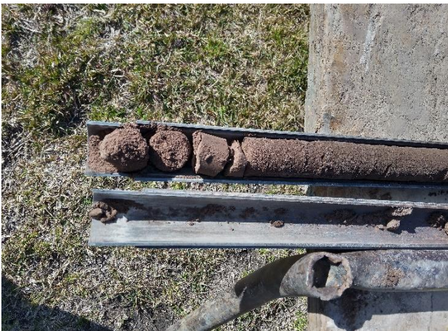
Photo 22: Borehole 5 SPT sample at 1.0m, Silty SAND.
