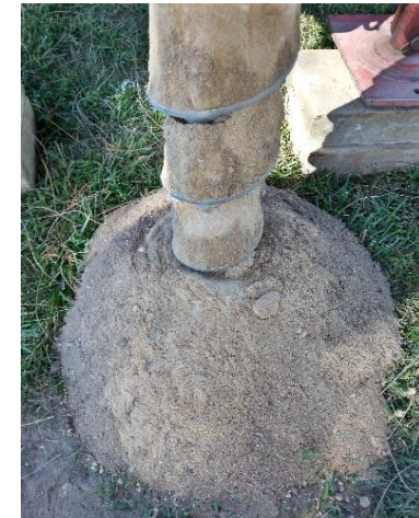
Photo 12: Borehole 8 spoil. Silty SAND.
