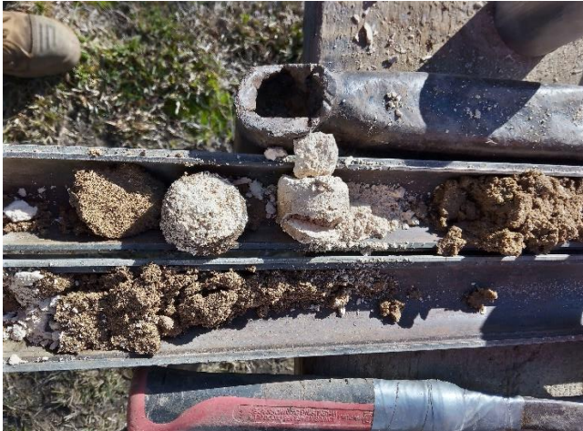
Photo 19: Borehole 4 SPT sample at 4.0m, Clayey SAND.
